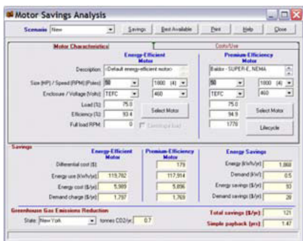
Figure 2: MotorMaster+ International provides an energy savings analysis feature to help users determine the "best available" motor to fit their needs.
